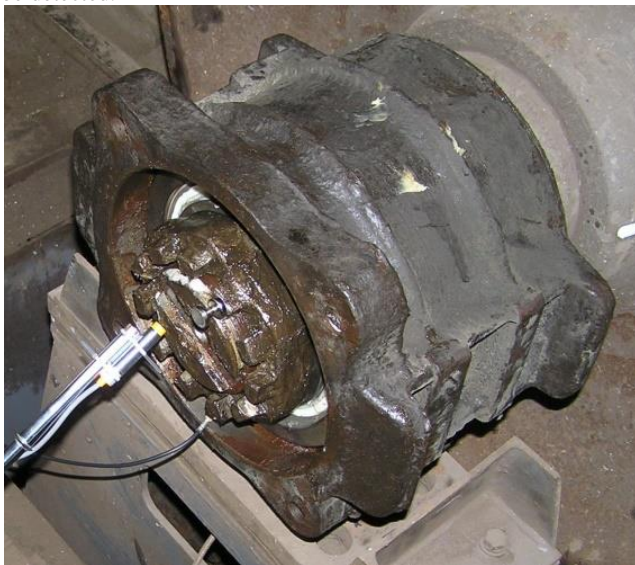
Fig. 21: Wheelset test rig
