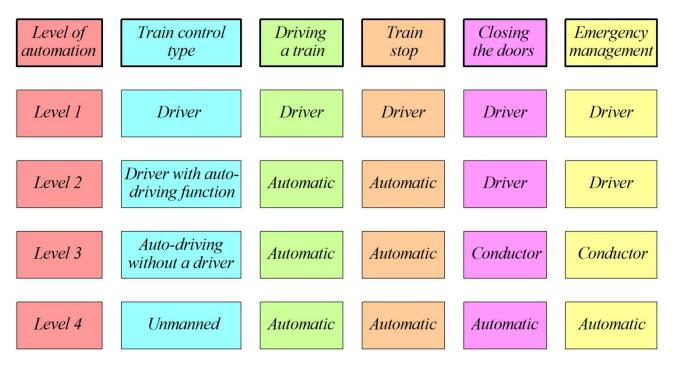
Fig. 1. Levels of railway transport automation
