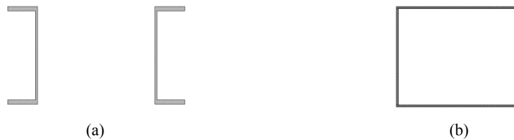
FIGURE 2. Cross-section of the center sill of the frame: (a) standard structure; (b) improved structure.
