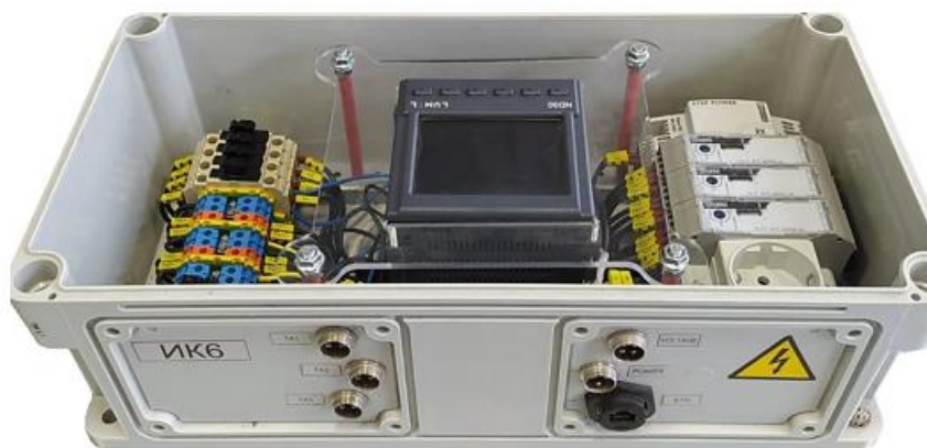
Fig. 1. Measuring set of parameters of the power supply network
